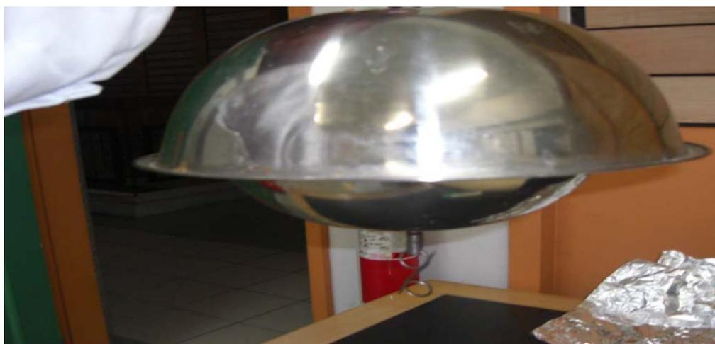
**Figure (26): The PAS sampler is ready for deployment onto monitoring site**
