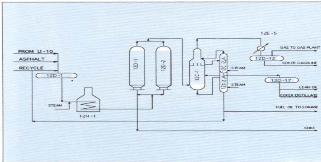
Figure (14): Delayed Coking Unit.
