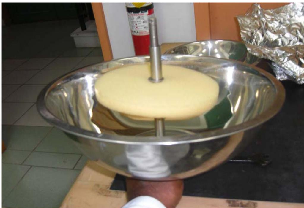
**Figure (25): Air sampler containing the PUF filter**
