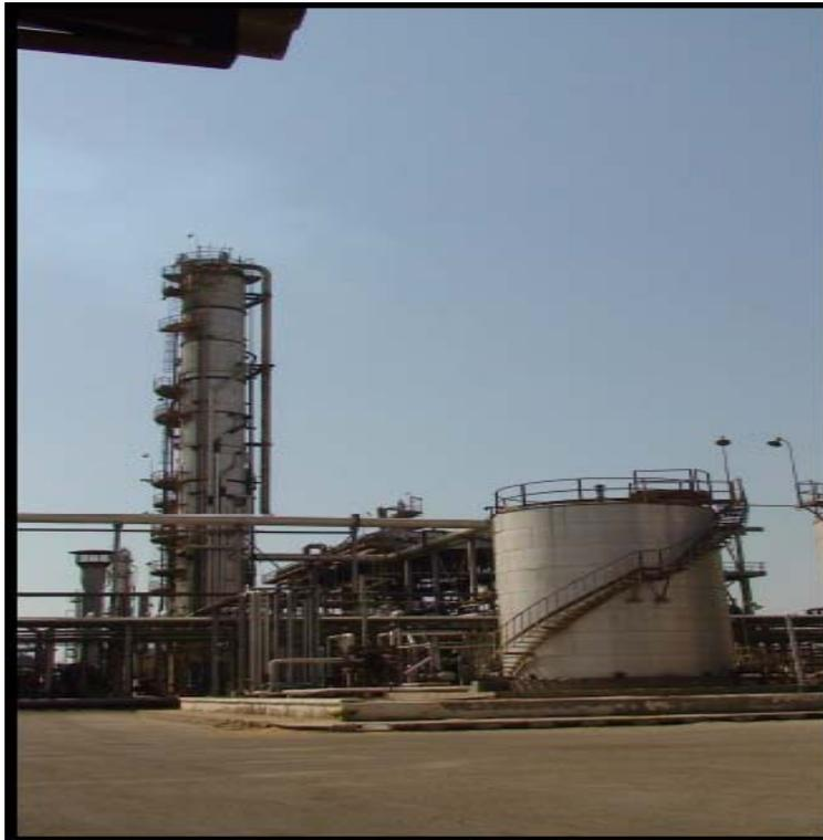
**Figure (32): Distillation unit**
