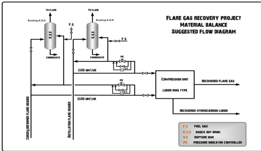
**Figure (21): Proposed scheme for the flare gas recovery project.**
