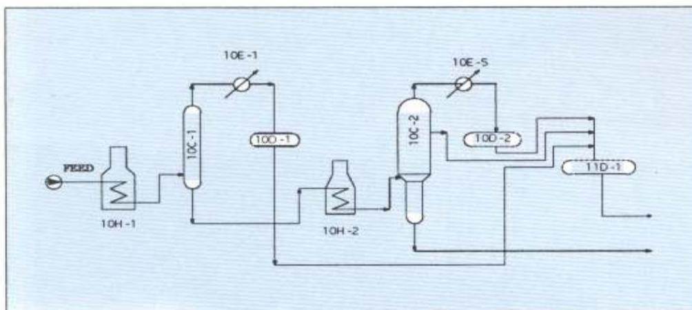
**Figure (13): Skimmed Crude Two Stages Distillation Unit.**
