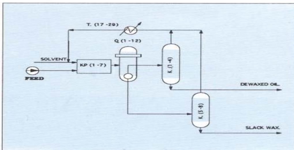
Figure (18): Dewaxing Unit.
