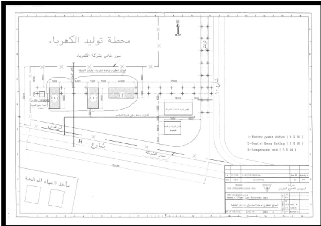
Figure (23): Proposed Position for the flare gas recovery Unit (Large Scale).
