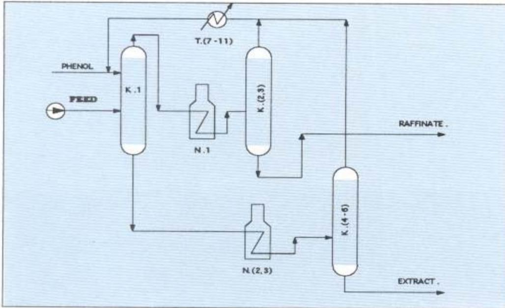
Figure (17): Phenol Extracting Unit.
