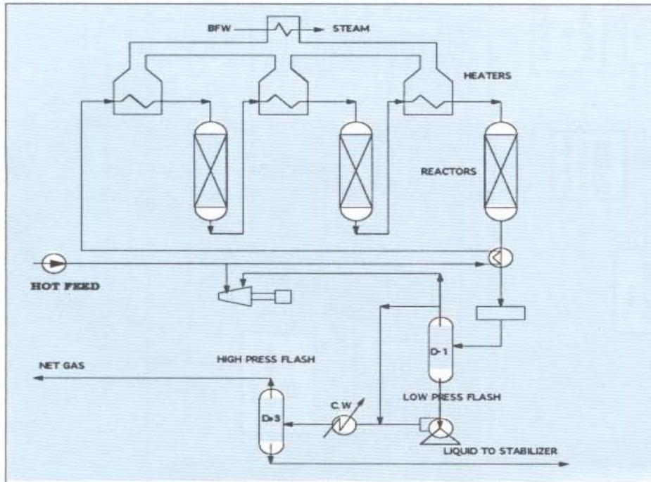
Figure (11): Catalytic Reforming Unit.
