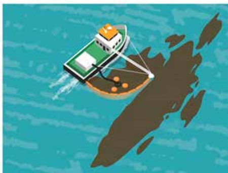
(Figure11) : Single-ship side sweep
