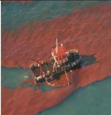
Side sweep vessel, with recovery system onboard
