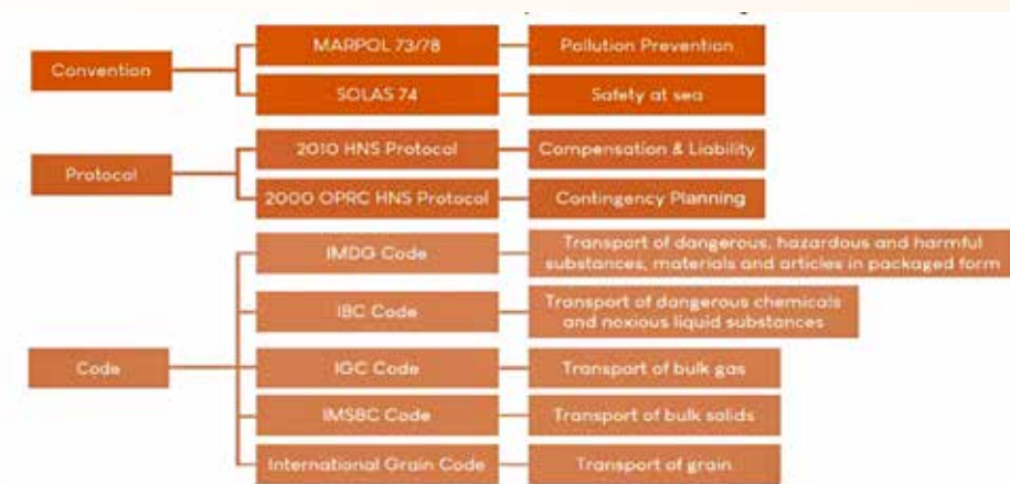
(Figure1) : IMO conventions, protocols and codes relevant for the transport of HNS at sea
