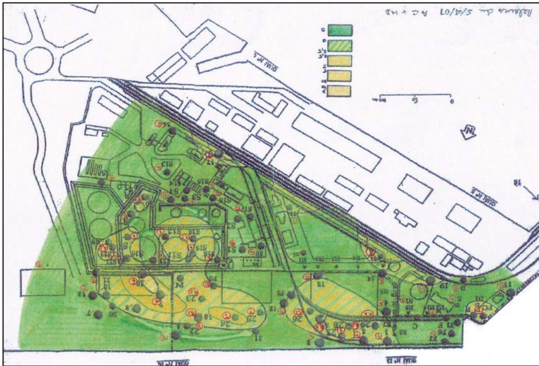
Figure 3. Map showing the thickness of the product in the wells (Floating thickness maps).
